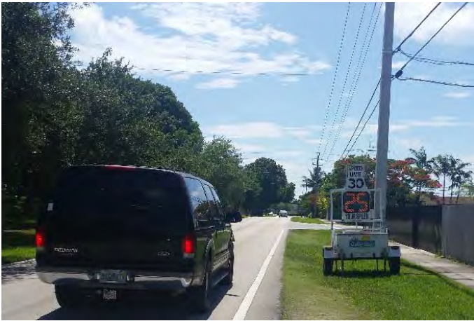
SW 186 Street east of Belmont Drive: A temporary mobile trailer-mounted radar was placed to inform drivers of their speeds and encouraging them to slow down.
