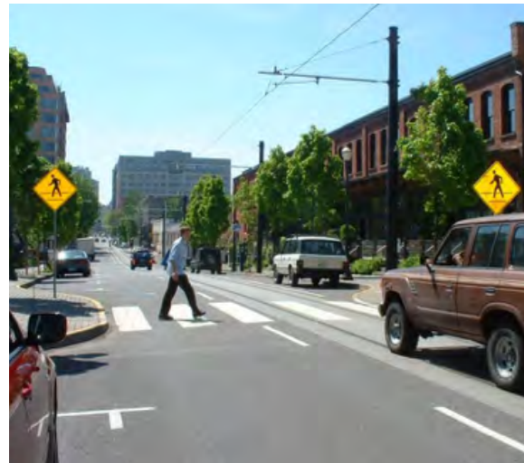
Curb extensions narrow crossing distances for safer crossings.
