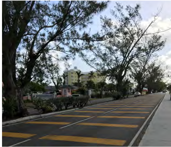
Pavement markings can be added to alert drivers that they are approaching a crosswalk.
