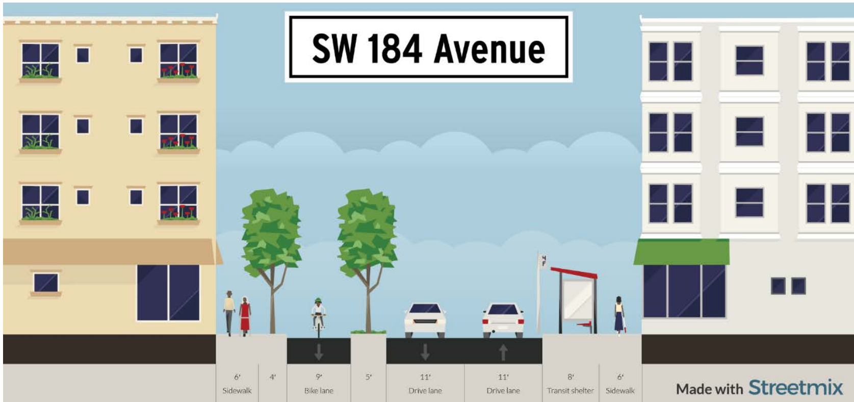
Figure 79: Proposed Street Section for SW 184 Street (Looking east from U.S. 1)
