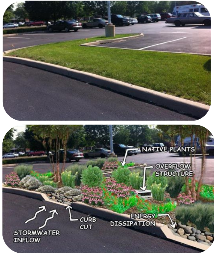
Figure 4.1.2. Bioretention – Before and After Parking Lot Island
