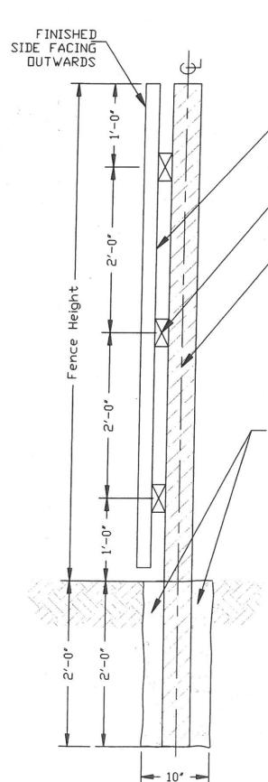
NOTE: ALL NAILS AND CONNECTIONS SHALL BE GALVANIZED
