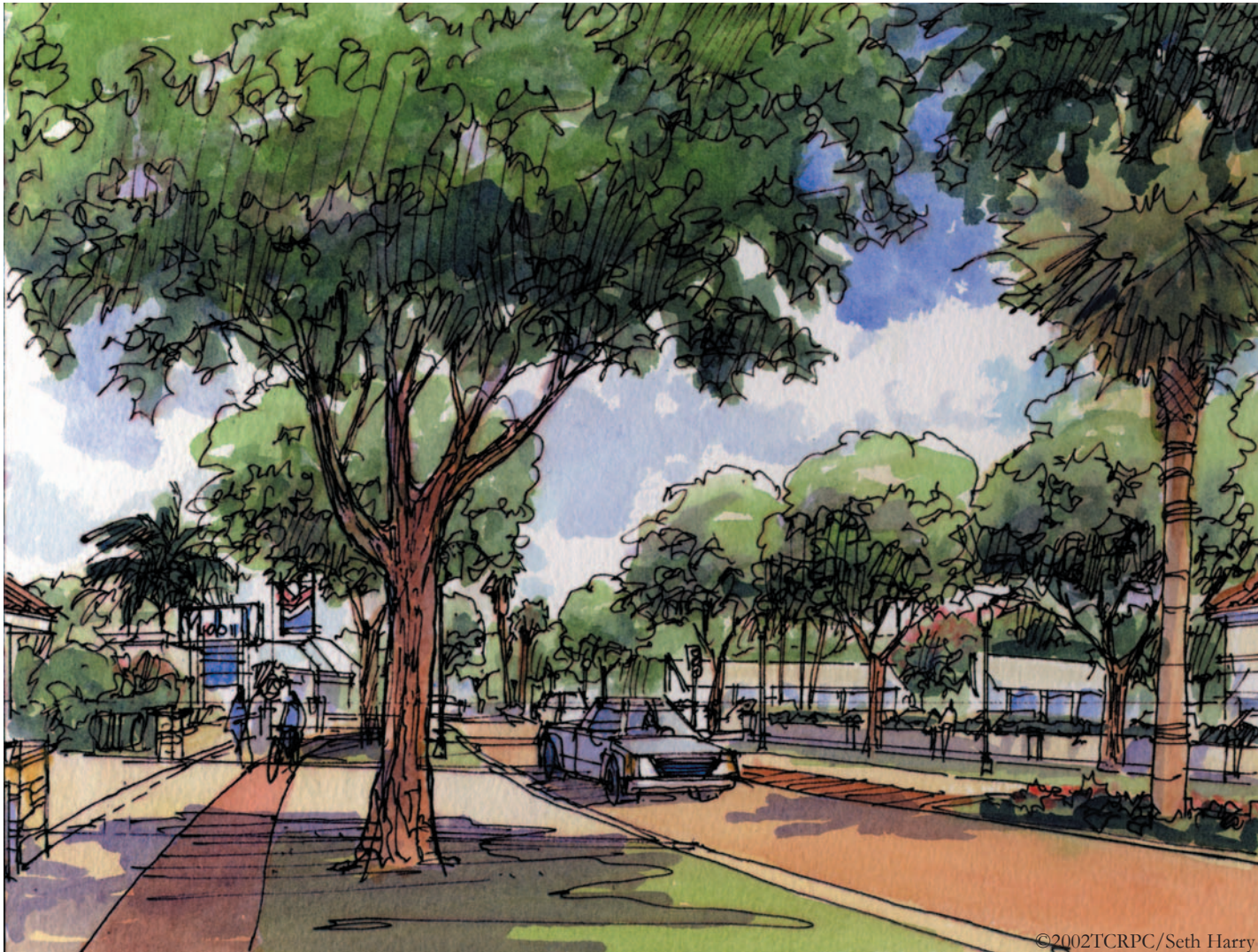
Looking north along the reconfigured section of Old Cutler Road showing the protected bike lane, spot medians and the textured turn lane.
